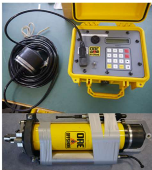
Acoustic release with SoundTrap hydrophone and external battery; Remote control deck unit; Schematic of deployed unit
