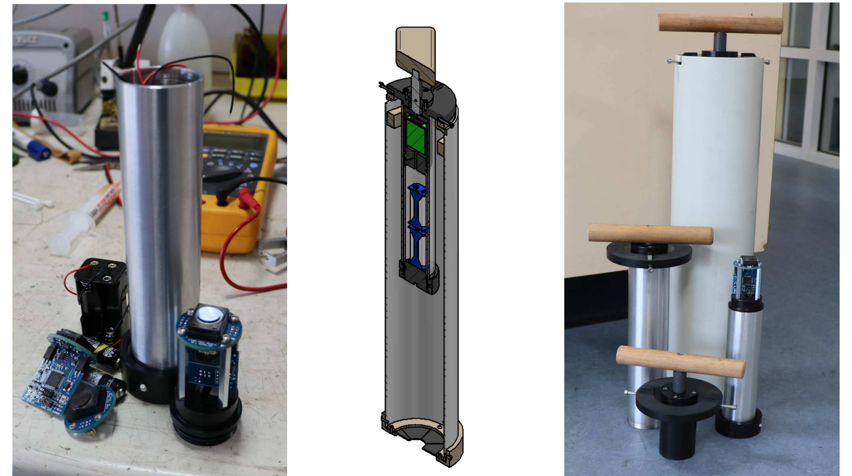
Figure 2: (Left) Various electronic components during manufacture and assembly. (Middle) Section view of assembled unit. (Right) Complete Frigatebird weight Logger and various subsystem assemblies shown on right.
