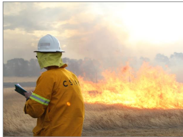
Figure 1 - Experimental grassfire burn to provide data for new rate-of-spread models.
