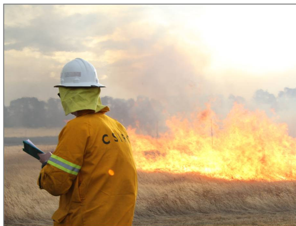
Figure 1 - Experimental grassfire burn to provide data for new rate-of-spread models.
