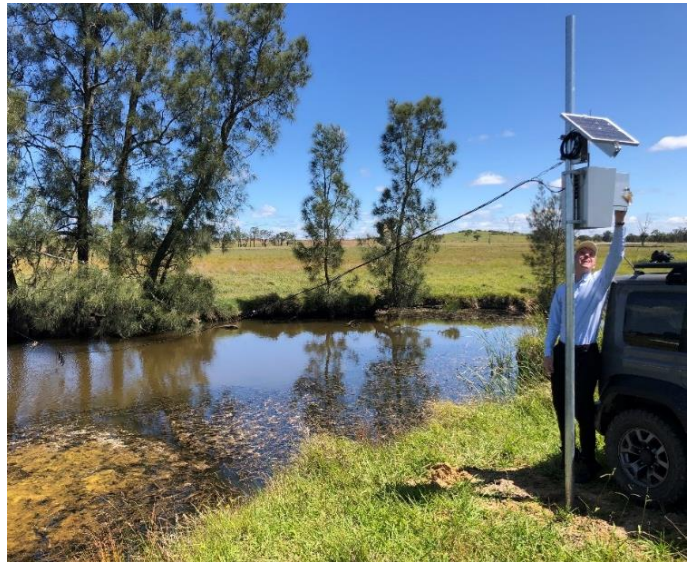
Figure 8. CSIRO water quantity and quality sensor installations. Left: sensor mounting within culvert (monitoring water flow onto SSP), Right: sensor mounted within the riparian zone, monitoring the third-order stream flow through SSP).
