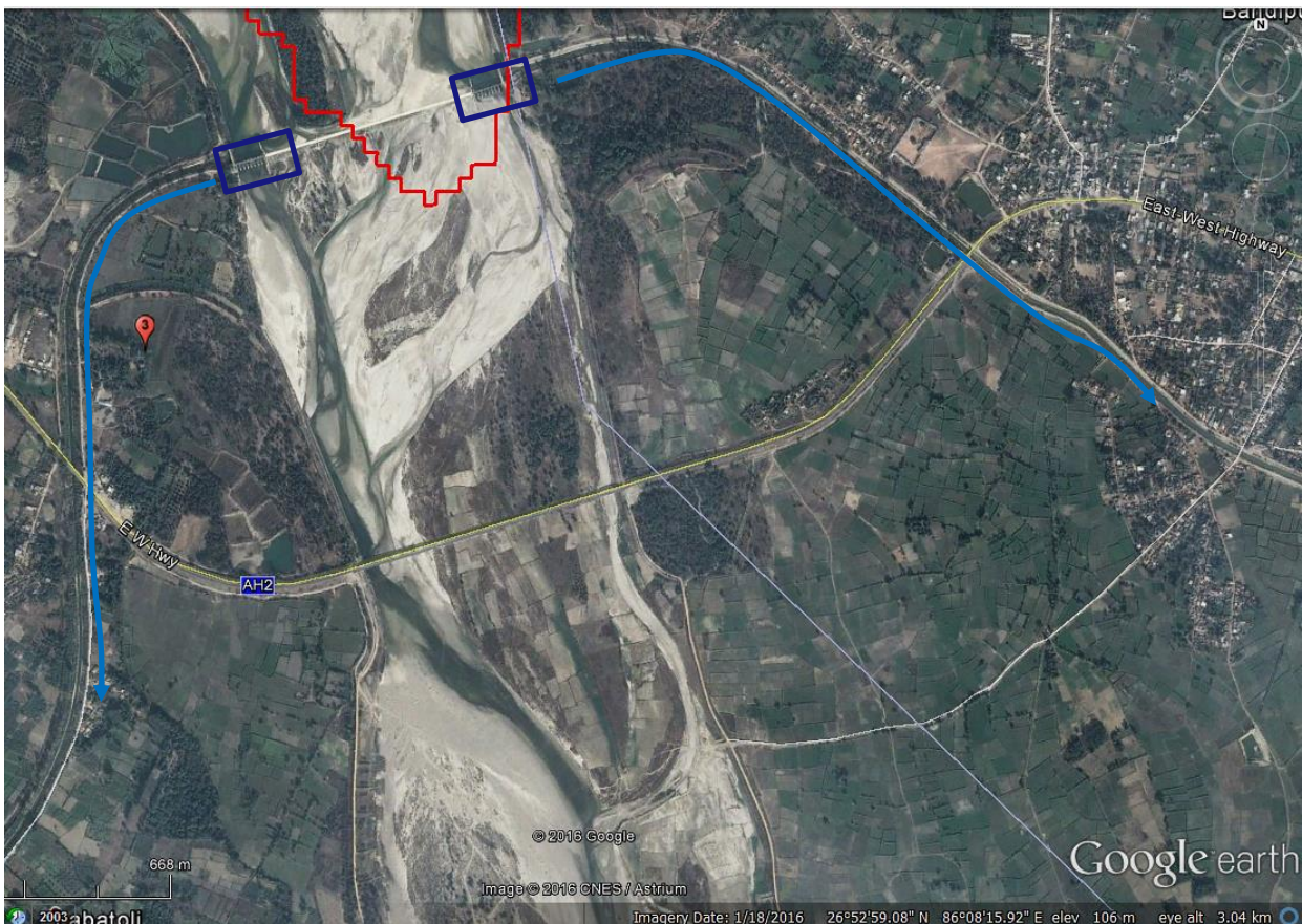
Figure 7 Satellite Image showing the two canals (blue lines) built to divert water from Kamala River for irrigation. The blue squares show the points where the water is diverted from the river
