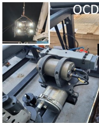
Figure 4-2 Two deployment methods were used to obtain water samples; Niskin bottles in a CTD rosette opened approximately 10m above the seafloor, and the OCD eDNA sampler attached to the deep tow camera system which was opened for the duration of a transect at approximately one meter above the sea floor. Water samples collected from the Niskin bottles included three replicate 1L samples and duplicate 10L samples, while an OCD sample combined the 1L of water remaining in the closed device with 1L of deionized water used to dislodge any remaining eDNA that could be embedded on the 100µm mesh net. The material and size of the filter membranes are indicated for each sample.
