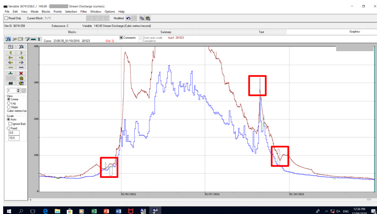
Figure 15: correction of discharges (gauging station on upstream side) calculated from best fit rating curves
