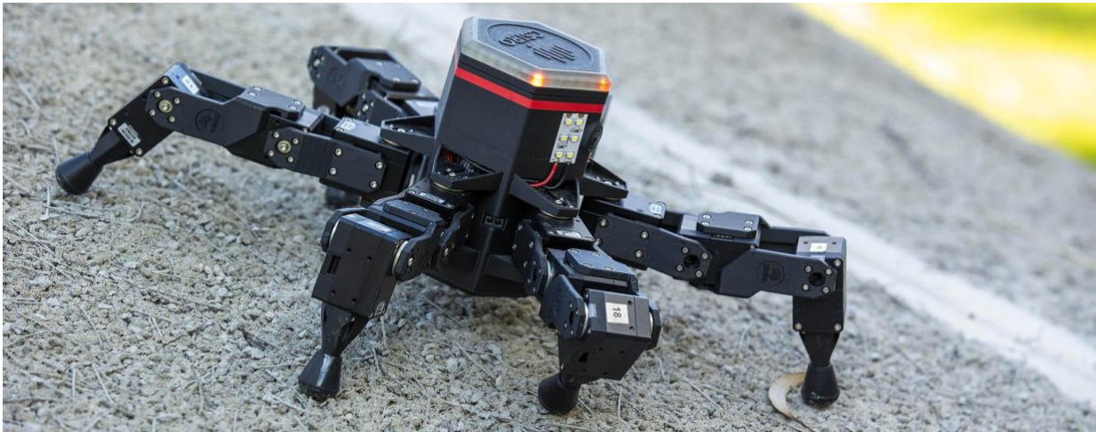
Data61's hexapod, Gizmo, draws inspiration from nature and can be used to inspect confined spaces.
