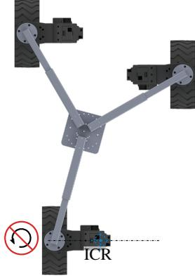
Fig. 8: Robot configured to align with the failed steering actuator on the back of a three-wheeled platform
