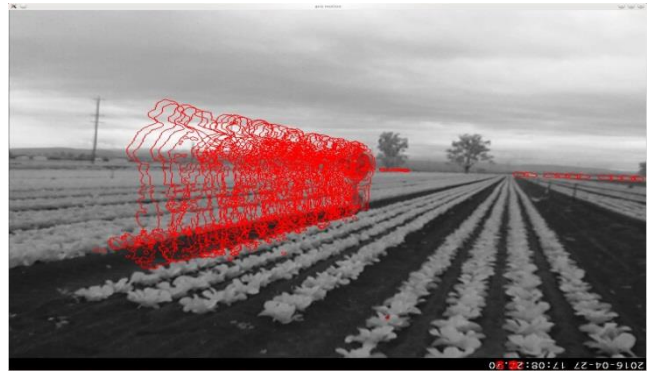
CSIRO system to detect moving objects in a Gatton lettuce crop – time lapse shows a person moving through the crop with cars in the background (red dots)
