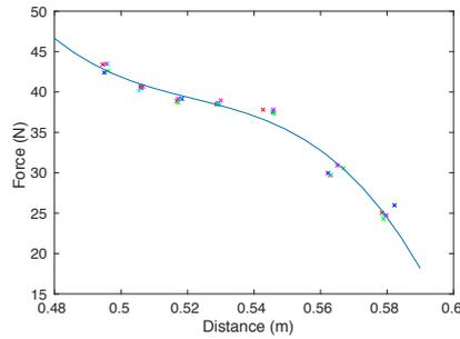
**Fig. 3.** Maximum force calculated at each probe for each movement iteration of the COM vs. distance from the probe point to the COM for multiple runs of the experiment (shown in different colours). A curve fitting was done to show the variation.
