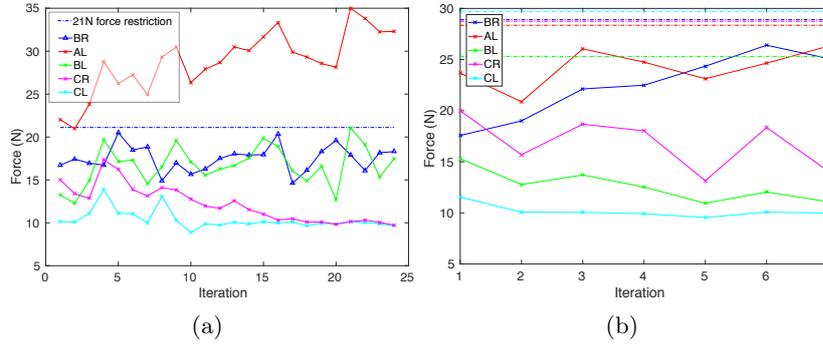
**Fig. 5.** Force profile with each iteration with force restriction set to 21 N is shown in (a) and the force profile of support feet with each iteration of COM movement with random force restriction on support feet is shown in (b). The dashed lines represent the force restriction for each respective foot.
