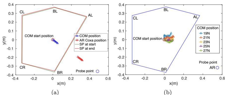
**Fig. 4.** COM movement during probing relative to the initial SP, with (a) showing COM movement with no force restriction on any foot and (b) showing COM movement for five trials, each with a unique force restriction set on the BR foot.
