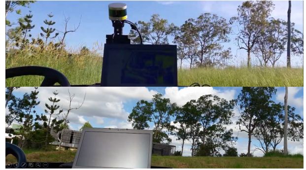
Fig. 7: Pictures taken approximately four months apart along the same track. The grass in the top pictures is approximately 1.5 m high and was freshly cut in the second photo. Localization and autonomous navigation were still working after the changes.
