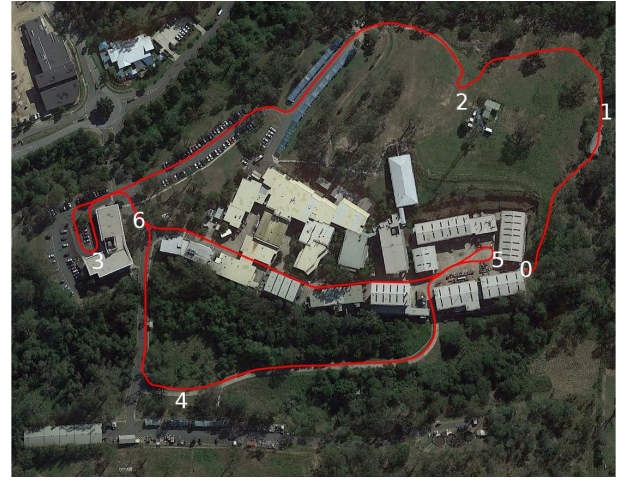
Fig. 6: Trajectory of an autonomous test run at QCAT overlaid on an image from google maps. The route was defined via six waypoints and spans a total length of 1.6 km.
