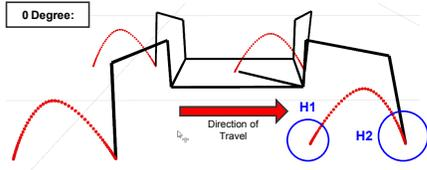
Fig. 7. Leg trajectories (in world frame) for  $0^\circ$  operation surface. H1: the beginning of the swing period where the tip magnet demagnetises and decouples from the walking surface. H2: the end of the swing period where the magnet is controlled to magnetise and adhere to the walking surface
