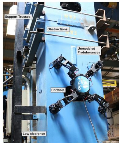
Fig. 1. Challenges faced by climbing robots in a typical industrial inspection scenario. The legged climbing robot, Magneto as shown in the scene, is built to explore open research questions of limited adhesion, whole-body planning and control, and complete coverage of complex 3D structures enabling the development of versatile climbing inspection robots.
