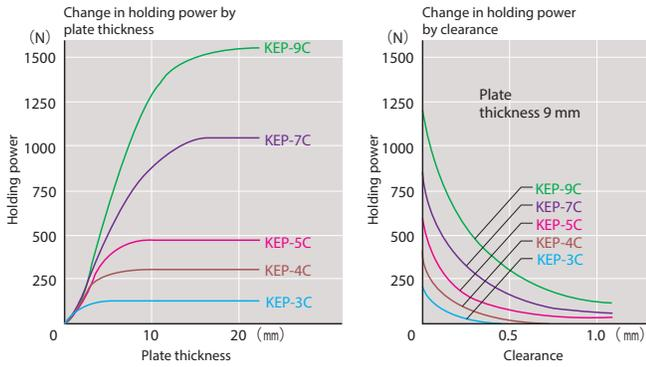
Fig. 3. Holding force of the Kanetec KEP magnet series vs plate thickness and clearance as provided in the manufacturer’s datasheet [20].
