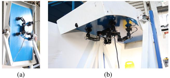
Fig. 12. Magneto traversing (a) vertical (90deg) and (b) inverted (180deg) surfaces
