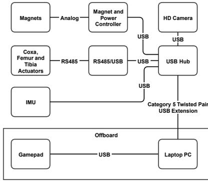
Fig. 5. System architecture of Magneto showing the sensing, actuation and controller connectivity
