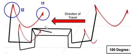
Fig. 10. Leg trajectories (in world frame) for  $180^\circ$  operation surface. (I1) Leg posing to minimise load on tip before initiating swing period. (I2) Leg posing to ensure magnet is in correct position/orientation at end of swing to make contact with, and adhere to walking surface.
