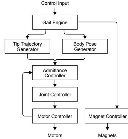
Fig. 6. Control architecture of Magneto showing the motor as well as magnetic adhesion control pathways.
