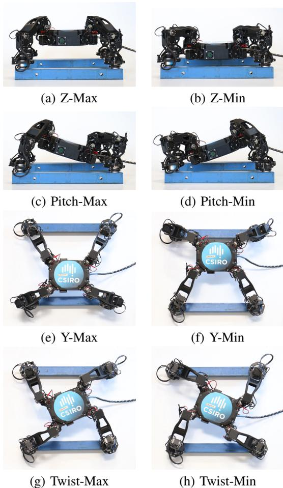
Fig. 11. (a-h) shows Magneto's limits of body posing for payload positioning.
