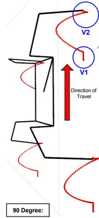
Fig. 9. Leg trajectories (in world frame) for  $90^\circ$  operation surface. (V1) Leg posing to minimise load on tip before initiating swing period. (V2) Leg posing to ensure magnet is in correct position/orientation at end of swing to make contact with, and adhere to walking surface.
