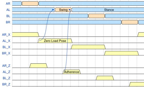
Fig. 8. Diagram detailing gait and leg pose timing example for traversing  $90^\circ$  plane. The Zero Load Pose and Adherence Pose periods are timed such that peak posing occurs during the start and end of the swing period respectively.
