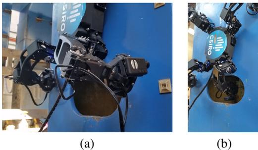
Fig. 17. Due to the design of its limbs and the control architecture, Magneto is able to seamlessly switch from locomotion mode to inspection mode. (a) shows Magneto's limb with a camera attached. (b) shows Magneto manipulating its limb to the interior of the structure through the porthole mid-climb.
