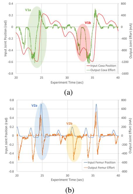
Fig. 13. Plots showing typical waveform of input joint position and resultant joint effort for Leg AR Coxa (a) and Femur (b) Joints during tests in a  $90^\circ$  operational mode. Highlighted are sections of the waveform which show the Zero Load Posing periods (V1a/b) and the Adherence Posing periods (V2a/b).
