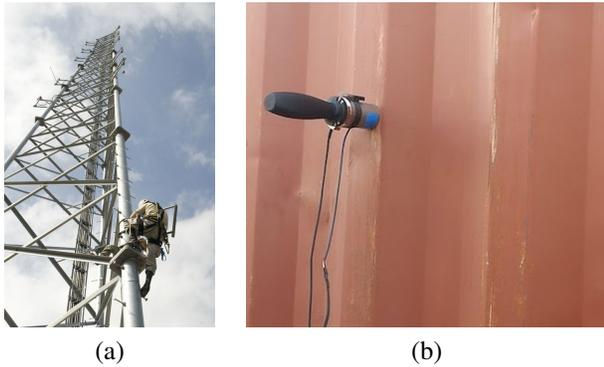
Fig. 2. Discontinuous surfaces of narrow width as seen in communication towers, seen in (a), and uneven surfaces seen on corrugated surface of a shipping container, as seen in (b), often limit the size of foot print available for adhesion. For scale comparison, a KEP magnet of width 40mm is attached to a ridge on the surface in (b). Wide footpads and tracks based robots become unusable for vertical locomotion on such surfaces.
