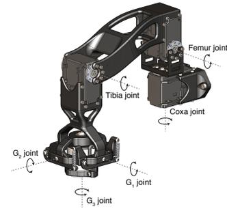
Fig. 4. CAD model of single leg showing all 6 DOF, 3 actuated and 3 passively compliant
