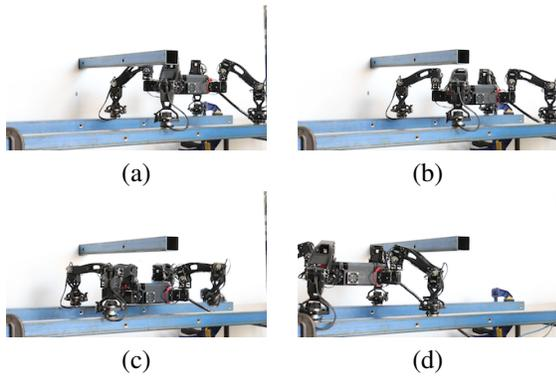
Fig. 16. Lowering body configuration to clear an obstruction with a maximum available clearance of 230 mm
