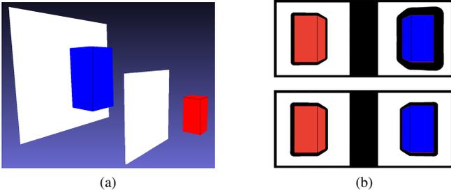
Fig. 5: A synthetic scene (a) is used to assess scale invariant properties of two kernels proposed in [9]. Figure (b) shows the projection of the visible points in (a) computed using the linear (top) and exponential inversion (bottom) kernels.
