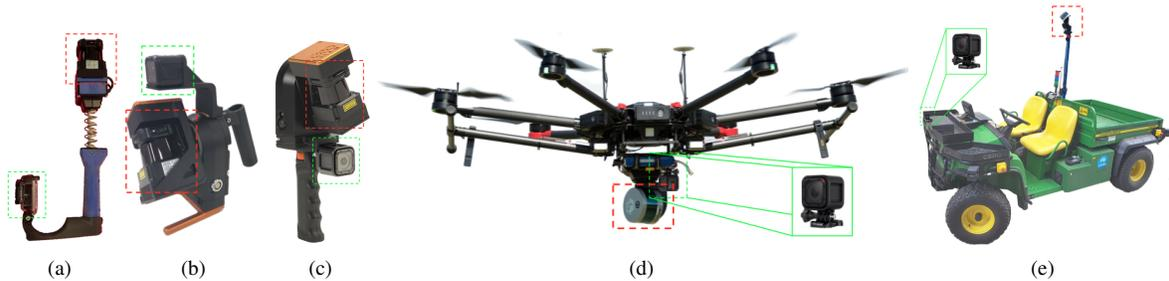
Fig. 1: Examples of mobile mapping devices with various lidar configurations, ranging from handheld (a-c), to aerial (d) and ground (e) platforms. The original lidar device is highlighted in red, while the added camera (which is not connected or synchronised to the lidar) is indicated by the green box. References for the lidar mapping devices: (a) Zebedee [2], (b) CSIRO Revo, (c) ZebCam [5], (d) Hovermap [6], (e) Gator [7].
