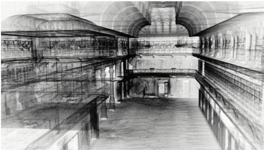
Fig. 2: Example illustrating the “transparency” effect in 3D lidar point clouds. This transparency can cause points that are occluded in the real world to be erroneously coloured when projecting an image on the points.
