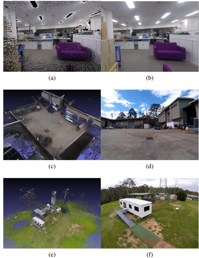
Fig. 6: Resultant colourised point clouds for (a,b) a hand-held system, (c,d) a ground vehicle, and (e,f) an aerial vehicle. The left column shows a view of the coloured point clouds and the right column shows captured camera frames.
