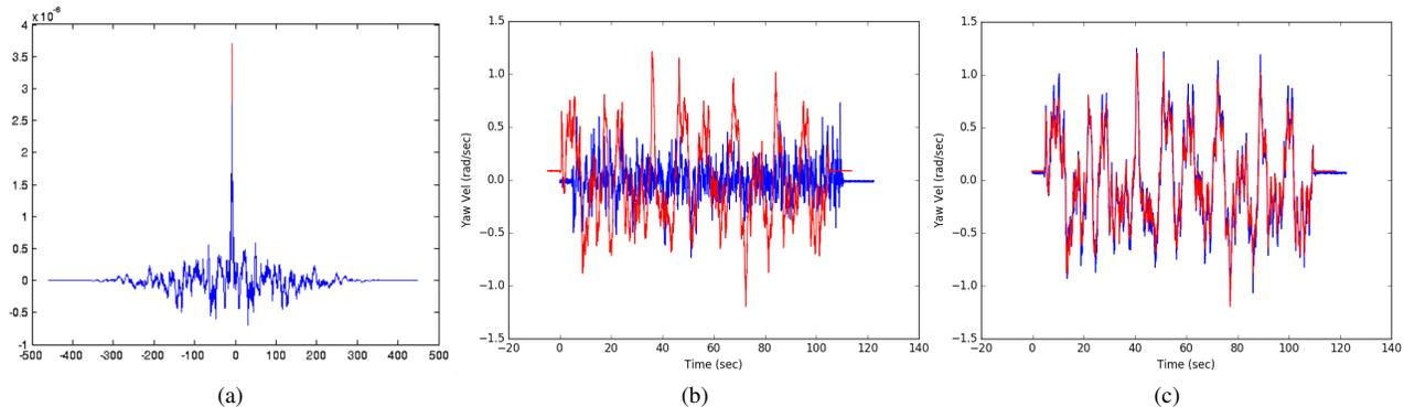
Fig. 3: Examples of (a) the cross-correlation output, (b) poor time synchronisation, (c) successful time synchronisation. The red and blue signals represent the yaw-rates of the camera and lidar, respectively.
