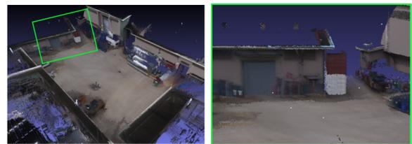
Fig. 7: Example illustrating the misregistration in areas of sharp 3D discontinuity and colour variation, such as the brown roof line against the blue sky (detail shown in the right image, corresponding to the green box on the left).
