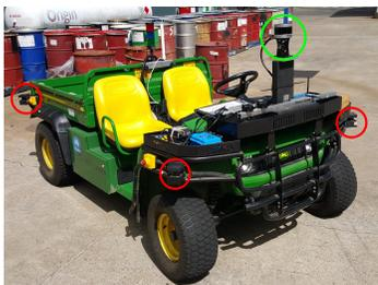
Fig. 3: The test vehicle is a John Deere Electric Gator. The 2D LiDARs are marked with red circles and the 3D Velodyne LiDAR with a green circle.
