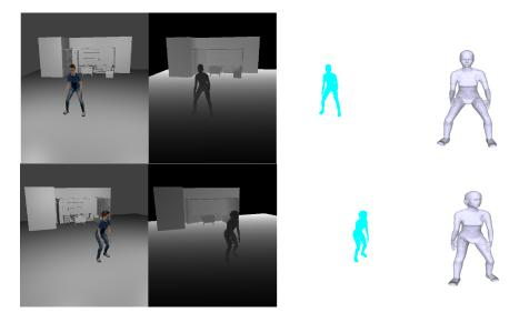
Figure 1: Some sample data from Subject2 is shown. For each row RGB image, depth image, foreground mask, and corresponding live geometry mesh is shown from left to right.
