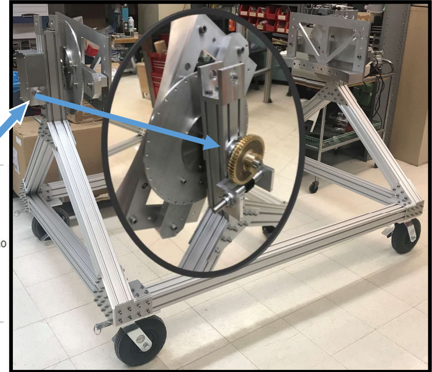
Crank-driven to rotate the cryostat in place
