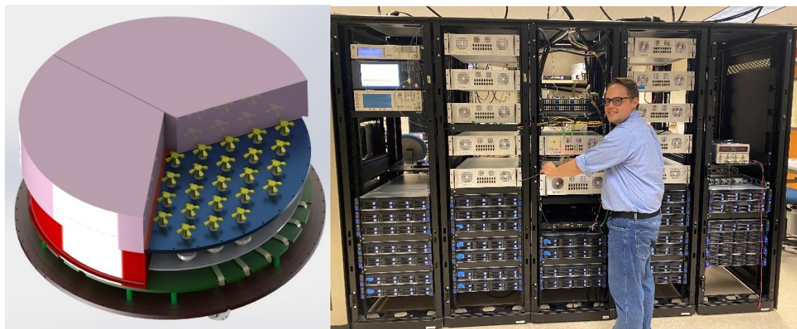
Figure 1. [Left:] ALPACA front end cryostat with the vacuum window and section of the RF clear foam removed showing the 20 K cryogenic array stage, the ground plane (blue), first 80 K stage (grey), radiation shield (red), and base plate (green). [Right:] Digital back end with 12 Xilinx ZCU216 RFSocFs, 27 HPCs, and 54 Nvidia A10 GPUs.
