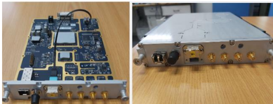
Figure 5. MeerKAT extension digitizer module.
