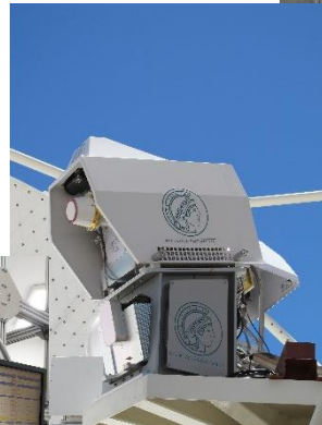
Ku-Band receiver for the SKAMPI Telescope in South Afrika
