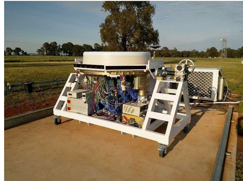
Fig. 14. Noise Temperature measurement from Absorber Y-Factor
