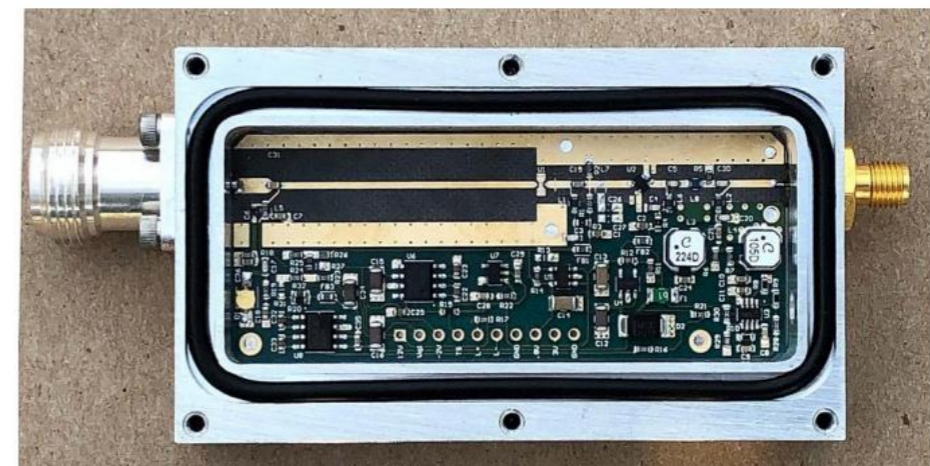
Low Noise Amplifier With 7-K Noise at 1.4 GHz and 25 °C. Sander Weinreb et. al 2021.
