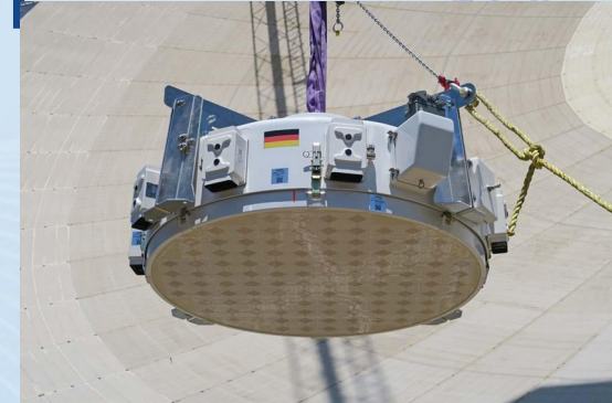
Top: CSIRO chequerboard PAF for the Effelsberg 100 m telescope during it's first installation (March 2017)
