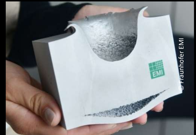
Effect of impact of a 1-centimeter aluminum ball traveling at 6,500 m/s on a solid aluminum plate with a thickness of 7.5 cm (Fraunhofer EMI)
