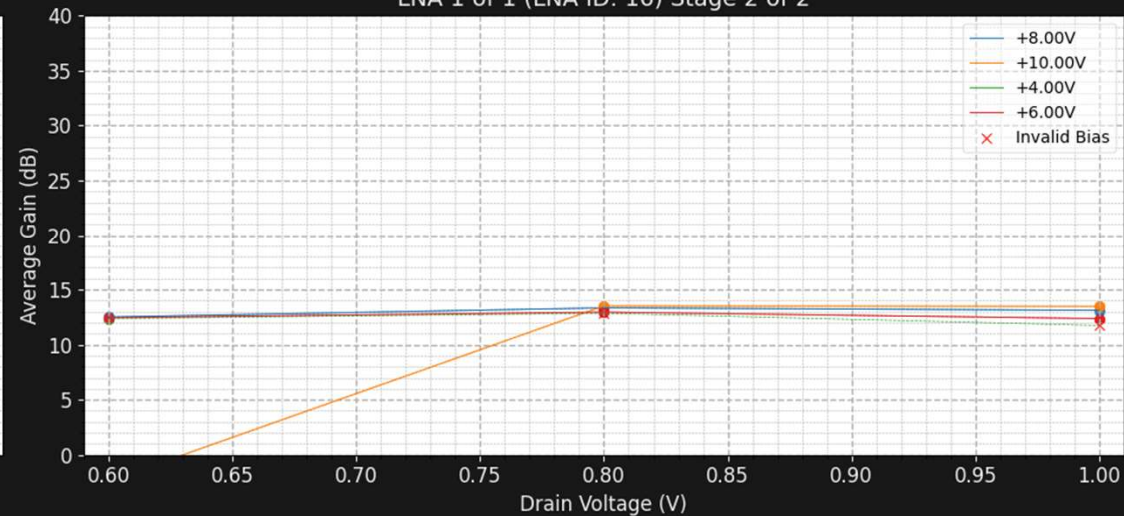
Average Gain (dB) Over Drain Voltages (V) LNA 1 of 1 (LNA ID: 16) Stage 2 of 2
