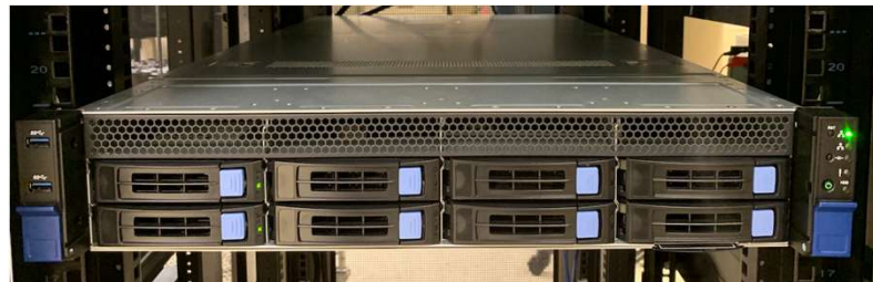
25x 2U Tyan Transport HX, AMD EPYC 96 GB DDR4 RAM, PCIe 4.0
