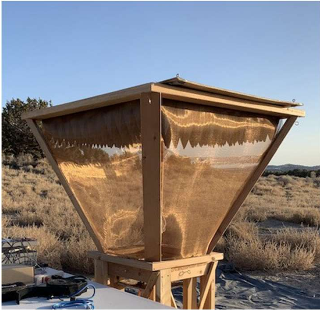
Ground shield with absorber foam (hot load)
