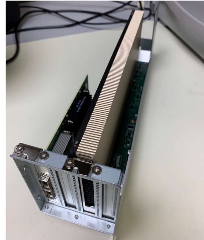
50x (2 per server) NVIDIA A10 GPU and ConnectX-5 dual-port InfiniBand EDR NIC
