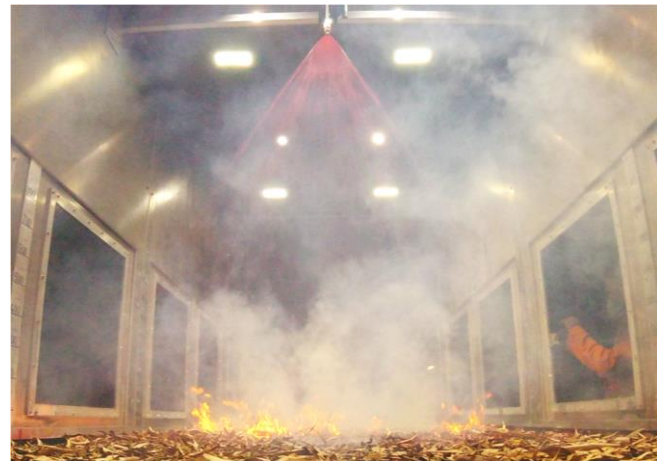
Figure 1. Retardant being sprayed onto the head of a standard laboratory fire (spreading toward the camera) during the appraisal of the direct suppression test.
