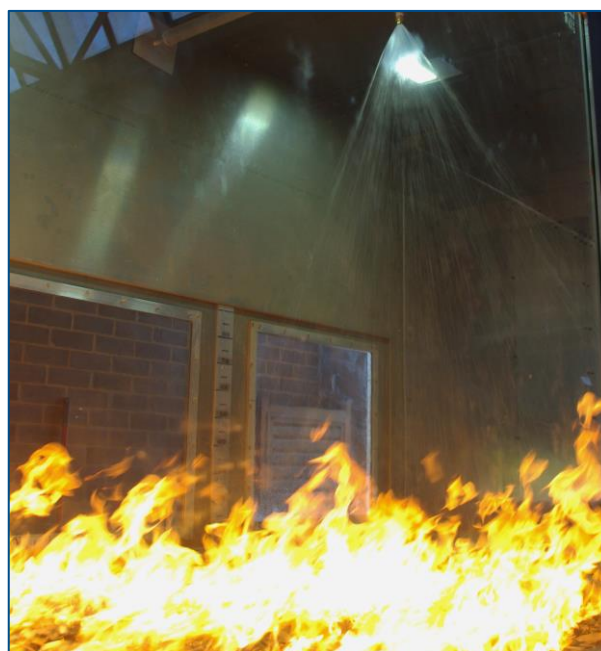
Figure 1. Laboratory scale testing of suppression chemical effectiveness on standard fires in the CSIRO Pyrotron.
