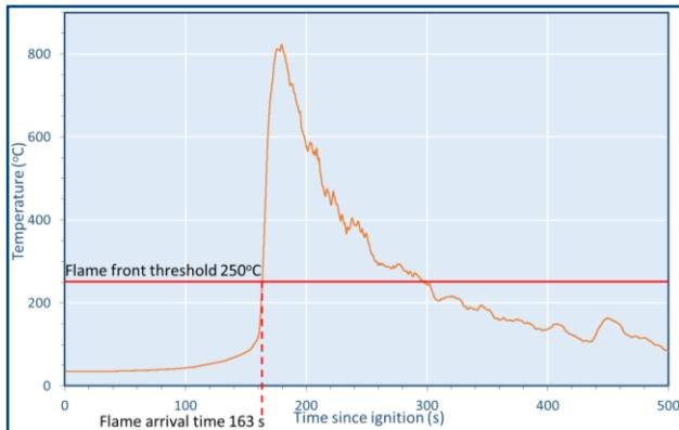
**Figure 2. Example of thermocouple trace from a fast moving fire in the Pyrotron. Time of fire arrival at the thermocouple is assumed to occur at a temperature of 250°C.**
