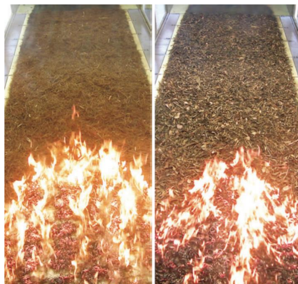
Figure 1. Oblique view from behind the ignition line of experimental fires burning in pine needle (left) and eucalypt litter (right) fuel beds in the CSIRO Pyrotron.
