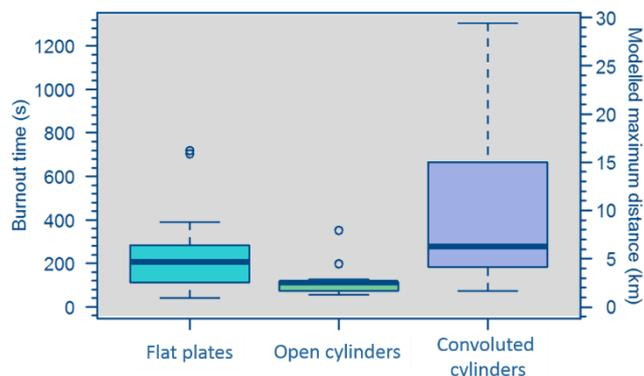
**Figure 3. Plot of burnout time and modelled maximum spotting distance. Outliers are examples of possible spotting distances.**
