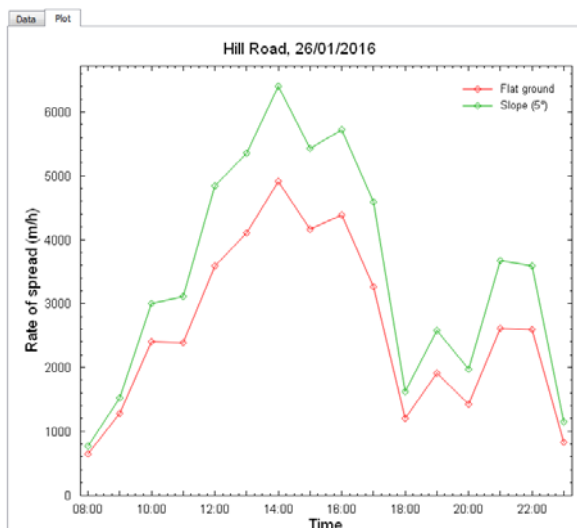
Figure 2. Screen shot of the fire behaviour graph showing diurnal variation in rate of spread for flat and sloped ground.
