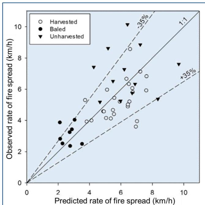
**Figure 2. Observed versus rate of fire spread predicted by the Cheney et al. (1998) grassland fire spread models with the natural pasture condition used for the unharvested crop condition, grazed pasture condition used for the harvested crop condition and the eaten-out pasture condition used for the baled crop condition.**
