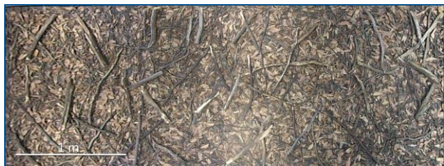
Figure 2. Plan view of an experimental fuel bed with 12 t/ha of woody debris scattered randomly over 10 t/ha of forest litter.
