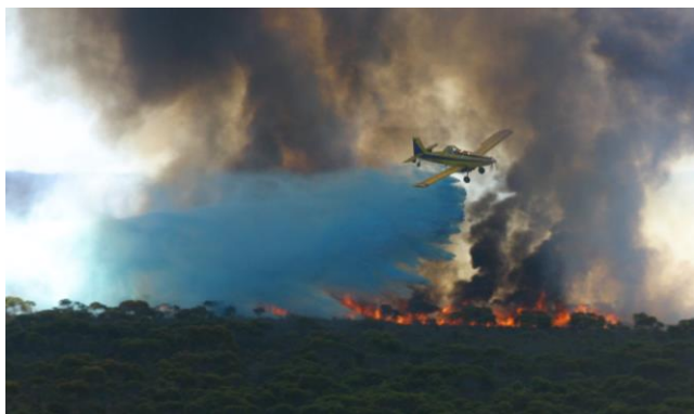
Figure 1. Gel being dropped on the head of a 6.9 MW/m experimental fire, which halted spread along 15 m of the perimeter for 6.5 minutes.
