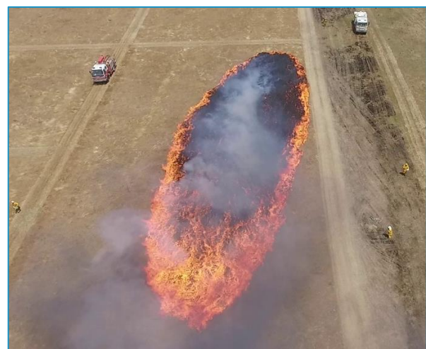
Figure 1. Aerial photo of a large experimental grass fire illustrating the changes in combustion behaviour around the perimeter as a result of different localised burning conditions.
