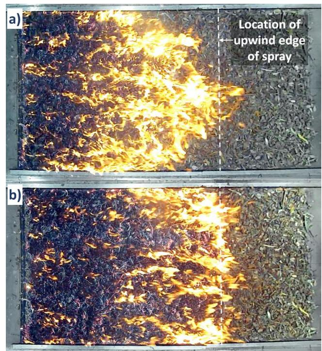
Figure 1. Overhead view of a suppressant evaluation fire (a) immediately before suppression and (b) during suppression application.
