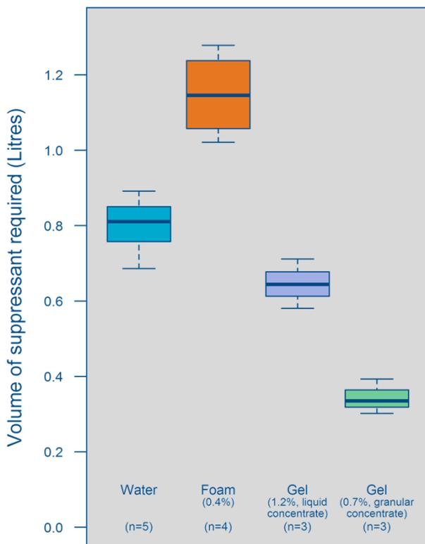
**Figure 2.** Plots showing the normalised distribution of the volume required for the extinction of standard fires using some example suppressants.
