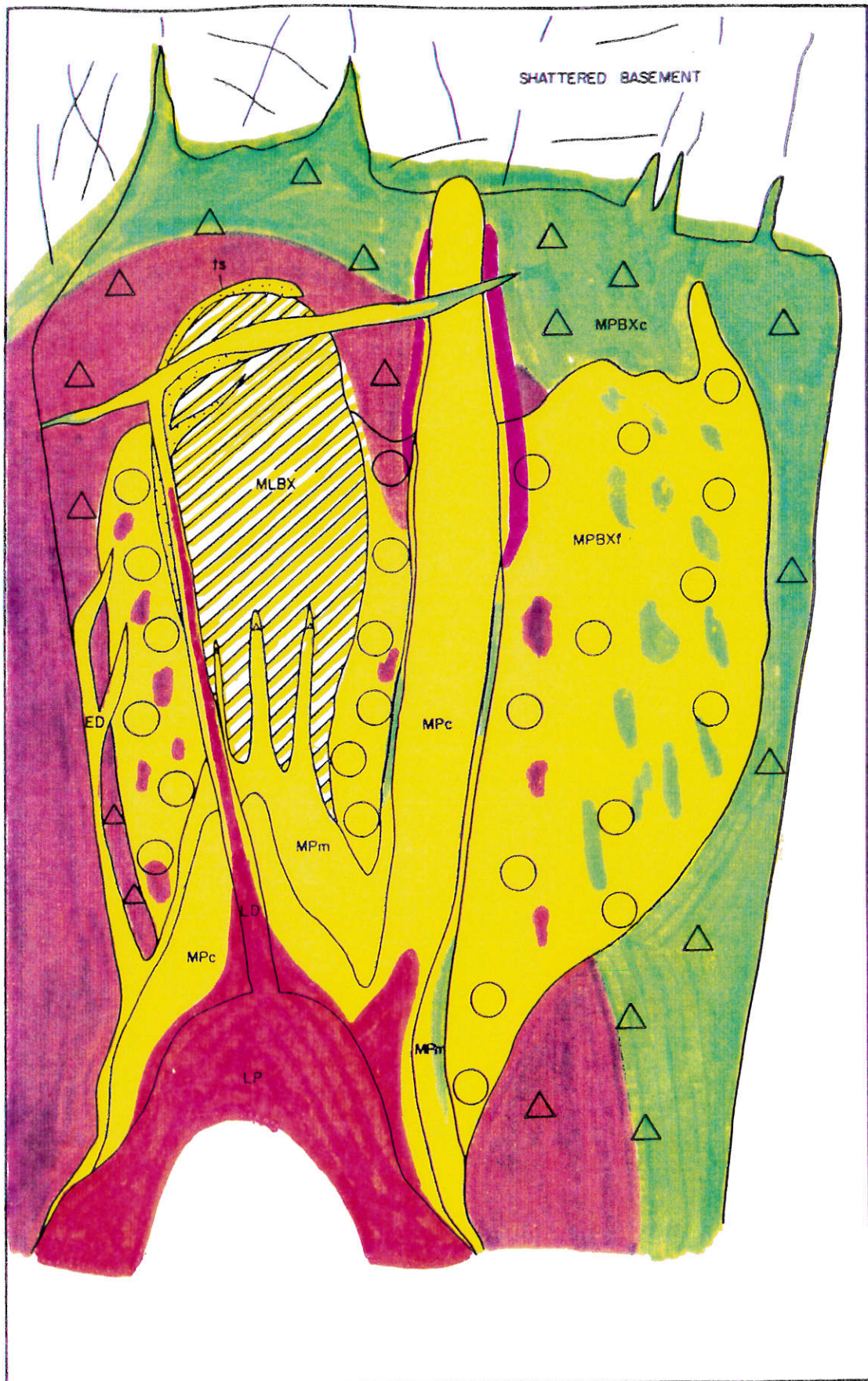
Schematic relationships between breccia units and intrusives in the Mount Leyshon Complex and distribution of alteration types. Green = propylitic; brown = biotite; yellow = phyllic; pink = K-feldspar; orange = albitic.
