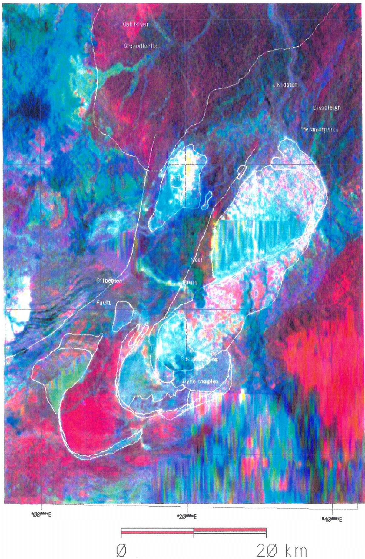
Fig.29. False colour composite image of regional radiometric compilation with K = red, U = blue and Th = green.
