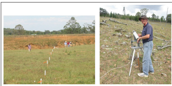
Fig. 10. 50mN line at Tallawang South (looking west) and the GETMAG rotating sensor head including the liquid nitrogen Dewar flask, which is mounted on a tripod at a 45^\circ angle (looking east, up the slope of the Gulgong Granite).
