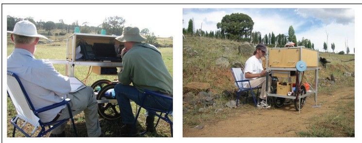
Fig. 11. Operating the GETMAG system via a notebook computer on a trolley, which carried control electronics, filters, and battery packs.
