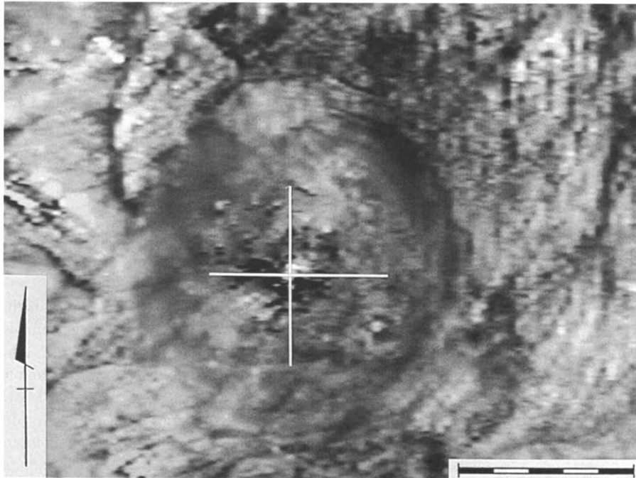
Fig. 5. Aeromagnetic image of the central part of the Acraman structure, showing a circular magnetic low \sim 20 km in diameter and a central high-amplitude dipolar anomaly. The east–west and north–south lines mark the positions of two profiles that pass through the central anomaly and which are modelled in Fig. 6. ER Mapper file: total magnetic intensity, greyscale, edges sharpened. Scale bar 10 km, north to top of image. Aeromagnetic data provided by MESA; see text for details of the aeromagnetic survey.
