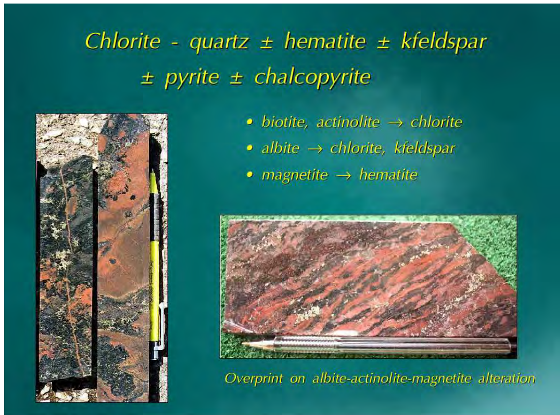
Fig.5.25. Magnetite-destructive chlorite-quartz \pm hematite \pm K feldspar \pm pyrite \pm chalcopyrite alteration typical of the Moonta area, South Australia, and similar to alteration associated with many IOCG deposits (Raymond et al. 2002)
