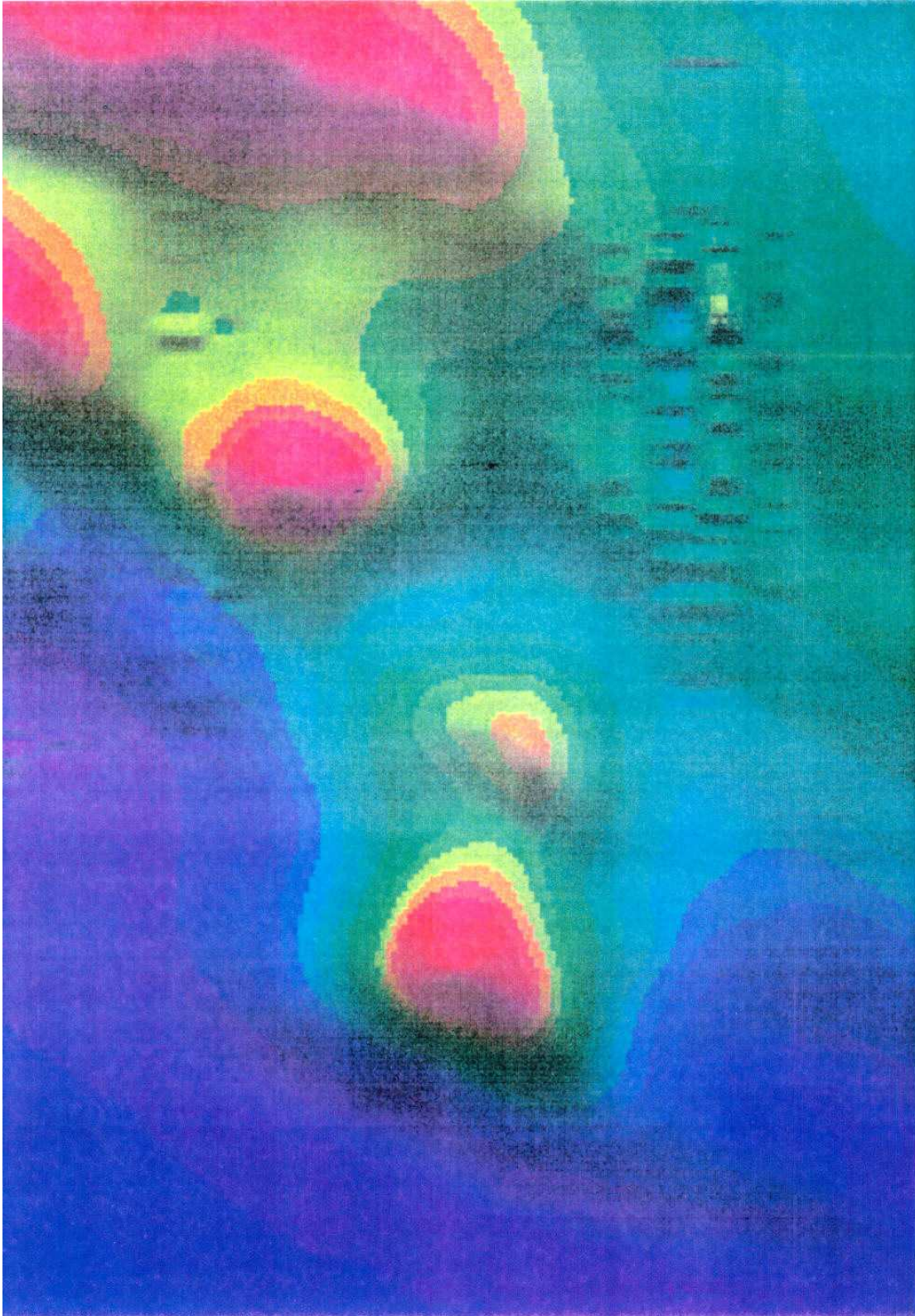
Fig.9.21. TMI image over the White Hill Prospect, Mount Woods area, Gawler Craton. Intense (up to 12,000 nT) magnetic highs are associated with magnetite-rich Cu-Au mineralised bodies ~100 m below the surface.
