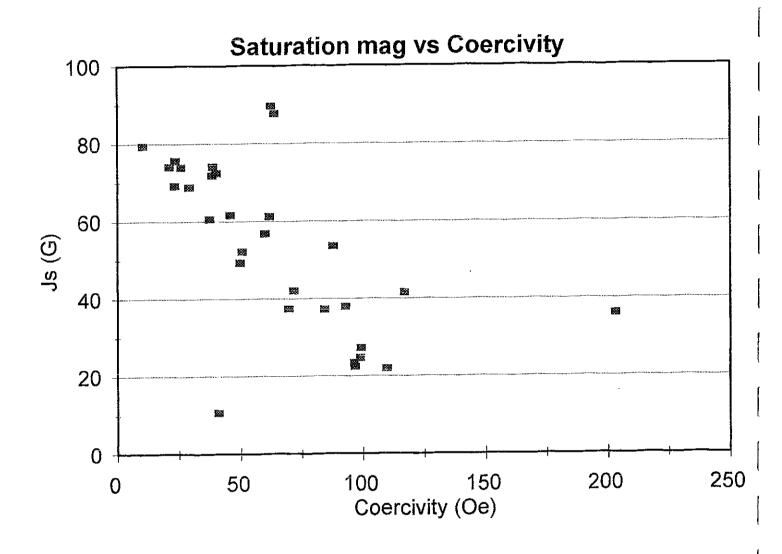
Figure 2. Plot of saturation magnetisation (Gauss) versus coercivity (Oersteds)
