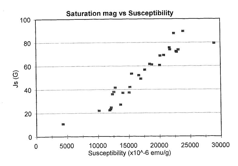
Figure 1. Plot of saturation magnetisation (Gauss) versus susceptibility (×10<sup>-6</sup> emu/g)
