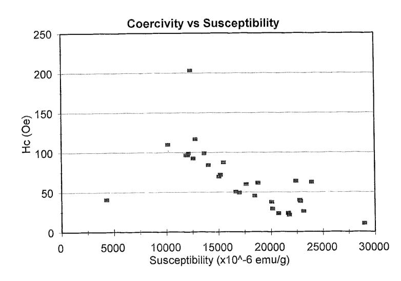
Figure 3. Plot of coercivity (Oersteds) versus susceptibility (×10-6 emu/g)
