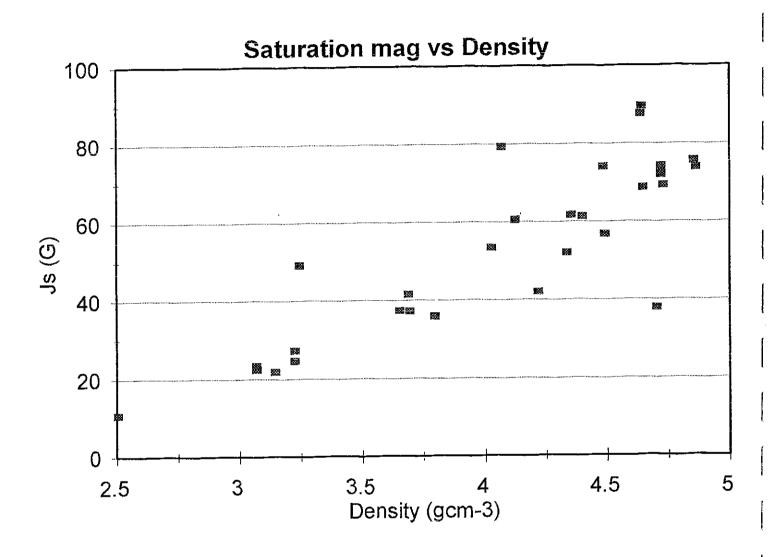
Figure 4. Plot of saturation magnetisation (Gauss) versus density (gcm<sup>-3</sup>)
