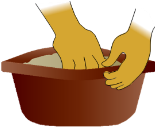
Figure 6. Mixing sub-samples by hand to make a composite sample
