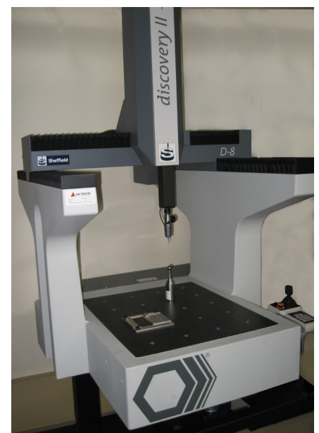
Coordinate measurement machine for surface profiling measurements.
