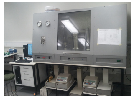
Core flooding rig for unconventional gas studies.
