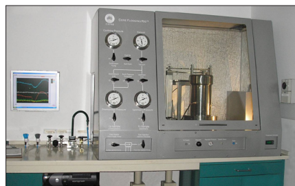
Facility for integrated laboratory characterisation of coal seam gas.
