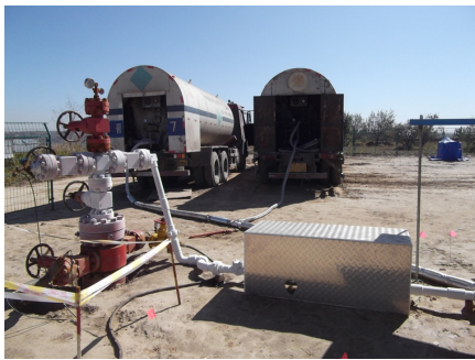
CO 2 injection during an enhanced coal seam gas field trial.
