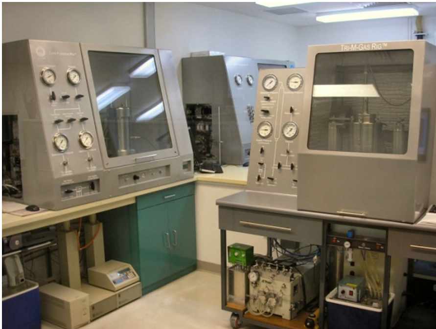
Core flooding facility to represent in situ conditions.
