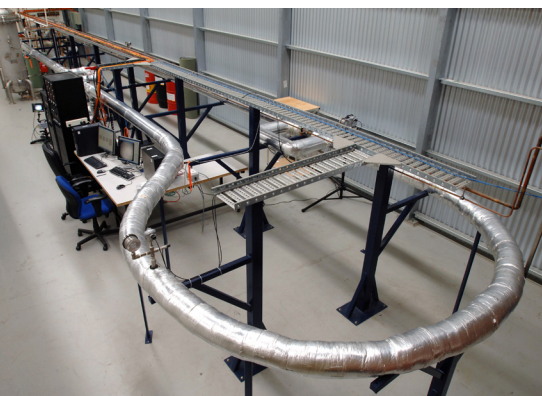
Layout of the hydrate flow loop.
