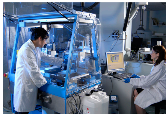
Materials library synthesis using Chemspeed robotic synthesis platform within the CSIRO High Throughput Centre.
