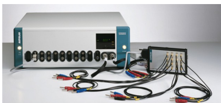
4-terminal dielectric/resistivity measurement is used in the frequency range from 1 mHz up to 10 KHz. An Autolab FRA30 potentiostat is connected to the in-house developed 4-terminal cell.
