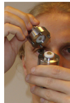
Using a coaxial transmission line cell the sample (white) is loaded between the inner and outer conductors.
